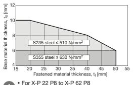
On higher steel grades, fastening with single nails (P8) may yield better results (e.g. less shear breaks) than fastening with collated nails (MX) due to better nail guidance.
