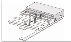
Typical application of X-HVB shear connector with steel deck, e.g. new construction.
