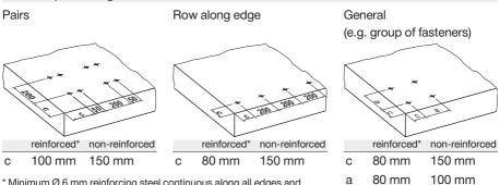
\* Minimum Ø 6 mm reinforcing steel continuous along all edges and around all corners. Edge bar must be enclosed by stirrups.
