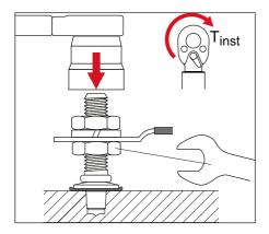
Hold the bottom nut with a spanner while tightening the upper nut.
