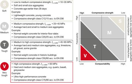
Note: f<sub>c. cube</sub> = compressive strength of concrete cube (150 mm edge length)
