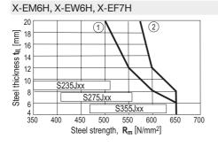
Fastener: X-EF7H-7-9 FP8 Setting tool: DX 6 F8, DX 5 F8, DX 460 F8
