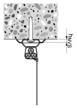
$\begin{array}{l} \mbox{Admissible fastener stand-off} \\ \mbox{$h_{\text{NVS, min}}$} &= 5 \mbox{ mm} \\ \mbox{$h_{\text{NVS, max}}$} &= 11 \mbox{ mm} \end{array}$
