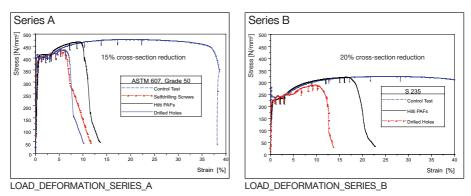
The test results were evaluated in terms of utilization as a measure of ultimate strength. Utilization is the ultimate load of a sample expressed as a percent of the ultimate load of the control test.
