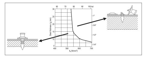
The application limit lines for long nails used to fasten wood to steel are plots of nail shank length  $L_s$  versus steel thickness  $t_{II}$ . Each line is valid only for one ultimate tensile strength of steel  $f_u$ . Attempts at working to the right of the limit line result in buckled nail shanks.
