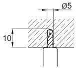
Pre-drilling with Hilti drill bit **TX-C-5/10B** until a ring on the concrete surface is visible.
