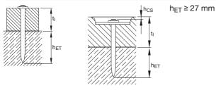
Fastener shanks length recommendation for fastening to steel
