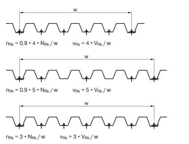
The same characteristic resistances can also be applied along supports at end-overlaps, if connection type "d" is not covered in the load table.
