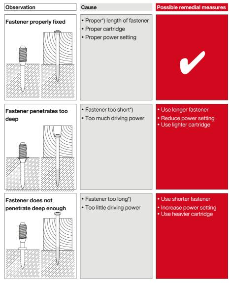
\*) Rule of thumb: The higher the compressive strength of concrete, the shorter the fastener Proper length (mm):  $L_s = 22 + t_l$  (compare, "Fastening Technology Manual" Part Product section)
