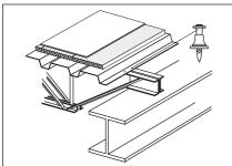
Roof decking (diaphragm design)
