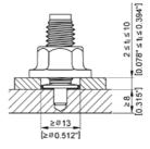
Fastened material hole Ø ≥ 13mm (0.51")
