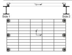
Grating element: X-FCS-R-3-25 Saddles connected to bearing bar: 2 Fastener: X-BT M8-15-6 SN 12 R Base material: S235 Base material thickness: t<sub>ii</sub> = 8 mm
