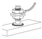
Recommended electrical Maximum allowable connectors: permanent current = 40 A X-BT-ER M10/7 SN 8 X-BT-ER W10/7 SN 8 X-BT-ER M8/7 SN 8 X-BT-ER M6/3 SN 8, X-BT-ER M6/7 SN 8 X-BT-ER W6/3 SN 8, X-BT-ER W6/7 SN 8 Note:
