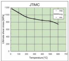
At 600°C, the CR500 material has 64% of its 20°C shear strength left. By comparison, standard fasteners have only 12% and structural steel only about 26%. The excellent fire resistance of the CR500 material alone justifies its use for some applications.
