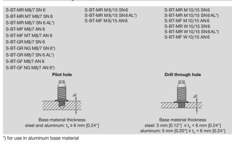
Thickness of base material corrosion protection layer ≤ 0.8 mm [0.0315"]. For thicker coatings, please contact Hilti. Base material corrosion protection layer
