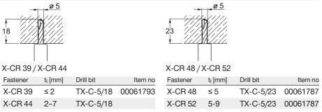
Details valid for C20/25 - C45/55 ( $f_{cc}$  = 25-55 N/mm<sup>2</sup> /  $f_{c}$  = 20-45 N/mm<sup>2</sup>)
