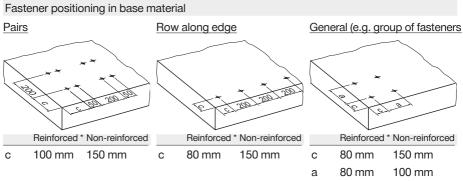
\* Minimum Ø 6 reinforcing steel continuous along all edges and around all corners. Edge bars must be enclosed by stirrups.
