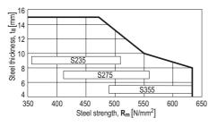
Application limit may increase in case of specific applications, like the fastening of wire mesh to steel, which is connected with X-CC U16 P8 fasteners. That wire mesh acts as reinforcement for fire protective sprayed coating. In such cases also different fastener stand-offs apply. Inquire at Hilti related with the use of X-CC U16 P8 in that specific application.
