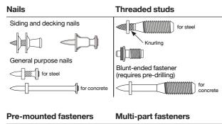
The nails used (also known as drive pins) are of a special type equipped with washers to meet the needs of the application and to provide guidance when driven. Threaded studs are essentially nails with a threaded upper section instead of a head. Composite fasteners are an assembly consisting of a nail with an application-specific fastening component such as a clip, plate or disk made of metal or plastic.
