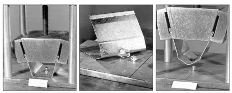
Pull-over test specimen at test start Sheet pull-over
