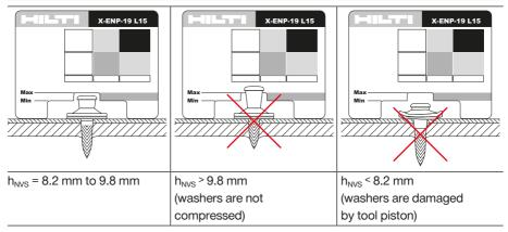
For multiple layer fastenings check piston mark on washer.
