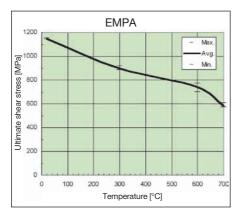
In Japan, similar tests were carried out by JTICM (Japan). These tests were done by driving a 4.5 mm diameter X-CR nail through a 6 mm steel plate into a second 6 mm thick steel plate and shearing the two plates. From the graph it is apparent that the results are nearly the same.
