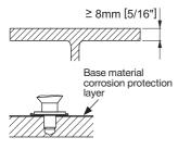
Where through penetration is not allowed\* Thickness of base material corrosion protection layer  $\leq$  0.4mm. For thicker coatings, please contact Hilti.
