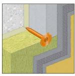
The XI-FV fastener is used to transfer wind suction loads acting on the thermal insulation composite system. The base material is normal weight concrete, which is either uncoated or coated with plaster or tiles. Coatings with plaster or tiles is often met if existing buildings are renovated and are improved with regards to their thermal insulation properties.
