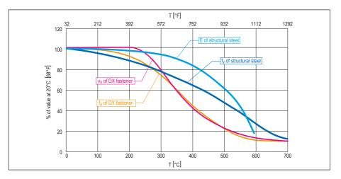
Up to about 300°C [572°F], the strength loss for DX fasteners is roughly proportional to the yield strength loss of structural steel. At 600°C [1112°F], DX fasteners have about 12% of their 20°C [68°F] strength left and structural steel about 26%. Since DX fasteners obtain their high strength through a thermal hardening process, the loss in strength at elevated temperatures is proportionally greater than for structural steel.
