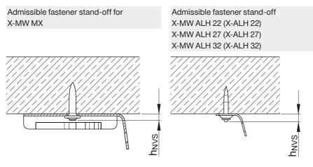
$h_{NVS, min} = 3 mm$  $h_{NVS, max} = 9 mm$
