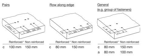
\* Minimum  ${\it \emptyset}$  6 reinforcing steel continuous along all edges and around all corners. Edge bars must be enclosed by stirrups
