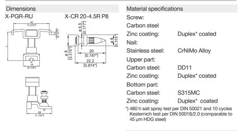
Recommended fastening tools DX 6 GR, DX 5 GR and DX 460 GR
