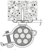
$h_{NVS, min} = 3 mm$  $h_{NVS, max} = 6 mm$
