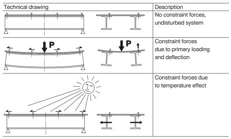
• When fastening large pieces of steel or aluminium, the possibility of shear loading due to forces of constraint must be taken into account in the fastening design. Allowance must be made for movement or, alternatively, forces of constraint must be taken into account in the design and maximum shear force limited by way of  $V_{rec}$ .
